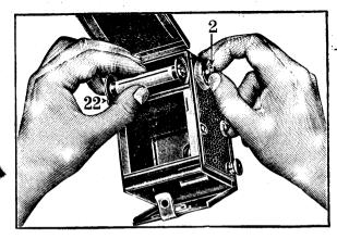
Fig. 9 Inserting the empty spool
