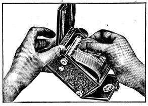
Fig. 12 Fixing the safety paper
