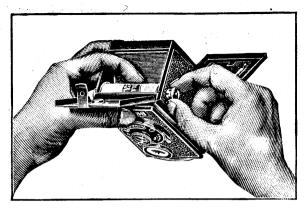
Fig. 10 enserting the full spool
