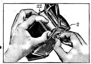
Fig. 14 Removing the exposed spool
