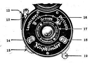
Fig. 5 Shutter with "Three Point" focussing
